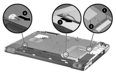
Disconnecting the SD Card Slot/Infrared Module and Speaker Cables from the System Board
